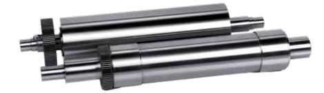
Rotometal supplies Anvil Cylinders as well as Support Rollers made from high quality tool steel. Depending on the customer needs, it can be induction hardened or through hardened up to 62 +/-2 HRC. Anvils can also be made as plus or minus cylinders to compensate for the difference in material thickness. Highest precision of execution ensures best possible pressure parameters, increases the lifetime, reduces the wear of dies, plates and press.
